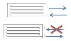
If the panel is installed at horizontal position, refrigerant inlet pipe should be connected into the bottom connection.
