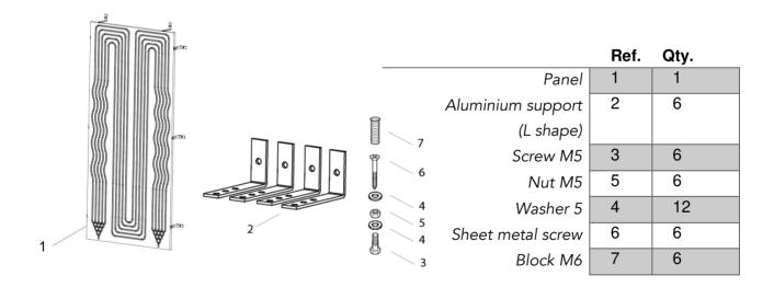
Anchor the panels using the lateral and front holes to the suitable surface.
