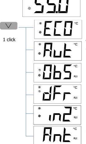
ECO Mode: Heating only by heat pump technology
