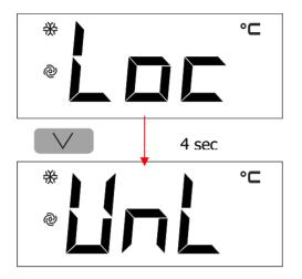
When 30 have elapsed without the keys being pressed, the display will show the "LOC" label and the keypad will lock automatically
