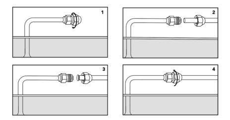
Then, join the suction line that comes from the panel to the coolant inlet of ECOHEAT, and the liquid line to the coolant outlet. The connections are threaded, if welding is needed, weld by oxyacetylene welding.
