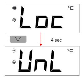
When 30 have elapsed without the keys being pressed, the display will show the "LOC" label and the keypad will lock automatically.
