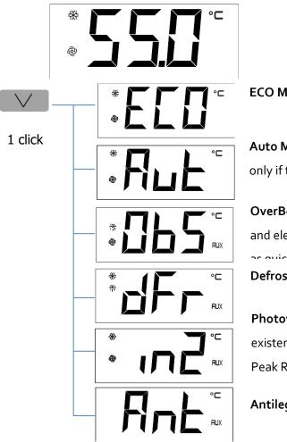
ECO Mode: Heating only by heat pump technology
