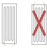
When the panel is installed in vertical position, always the inlet and outlet connection has been at the bottom.
