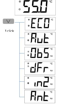
ECO Mode: Heating only by heat pump technology
