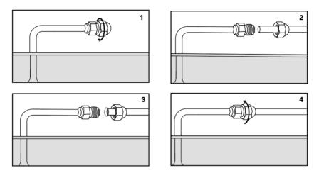
Then, join the suction line that comes from the panel to the coolant inlet of ECOHEAT, and the liquid line to the coolant outlet. The connections are threaded, if welding is needed, weld by oxyacetylene welding.
